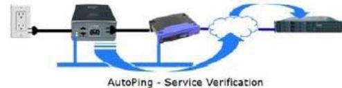
AR monitors a network device, and powers up an alarm or redundant system when there is no response. Ideal for Hot Standby Servers, Environmental Control, Alert for any network failure.
