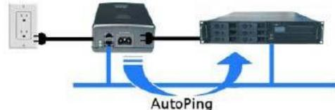
**Service monitor:** AR is installed with the device to be rebooted, but pings a remote host to test the communication channel. Ideal for DSL/Cable Modem verification.
