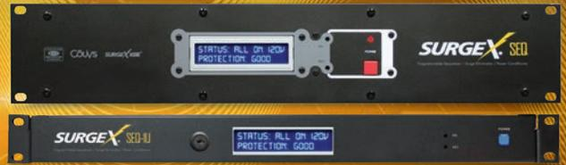
When electronic equipment must be powered up or down in order, rather than simultaneously, sequencing is needed. In AV systems, sequencing is often necessary for controlling power distribution to avoid pops and hissing sounds, along with excessive inrush surge currents that can trip circuits.
