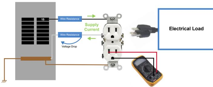
Figure 4. N-G Voltage caused by increased Wire Resistance
