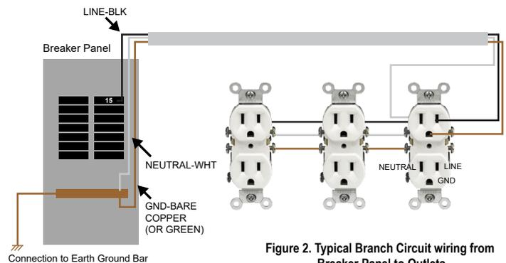
Figure 2. Typical Branch Circuit wiring from Breaker Panel to Outlets
