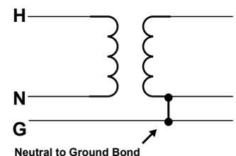
In addition to cancelling N-G voltages due to insufficient wire sizes and load imbalances in systems that share the NEUTRAL connection, it has the added benefit of cancelling out common mode N-G noise voltage created by Electro-Magnetic Interference and Radio Frequency Interference (EMI/RFI). Using an isolation transformer is a good practice in professional and residential audio/video systems requiring a very low noise floor to enhance performance.
