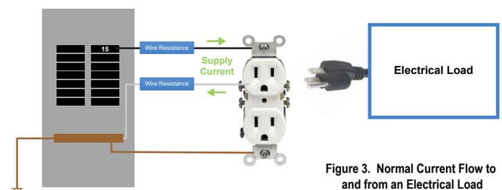
Figure 3. Normal Current Flow to and from an Electrical Load
