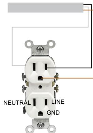
Figure 1. Wiring of a standard NEMA 5-15 Outlet
