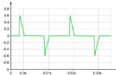
While the voltage waveform in power distribution is generated as a sine wave, the current draw by an electronic load may or may not be sinusoidal. Purely Resistive loads will pull current in a
