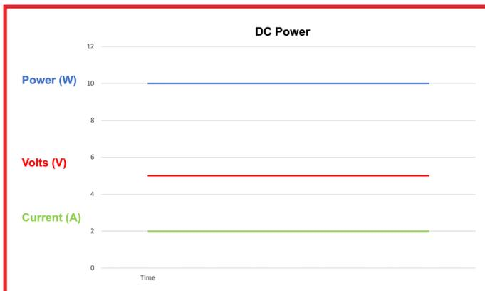
However, in an AC or Alternating Current circuit, calculating the power consumption is much more complicated. While DC voltage is constant, AC Voltages are constantly varying in a sinusoidal pattern. As you can see from the graph below, some electronic loads pull current at different points along the voltage waveform. Purely resistive electronic loads pull current in a sinusoidal pattern that "line up" or are in step with the voltage
