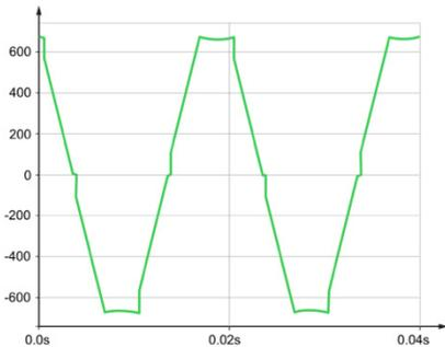
Voltage waveforms associated with Power distribution start out sinusoidal but are often not perfect by the time they get to the point of use. A common issue in AC electrical systems is called “Flat-Topping”. Flat-Topping occurs
